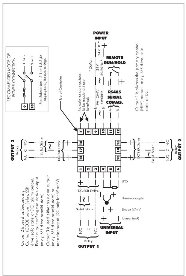
Figure 1-4 Rear Terminal Connections
